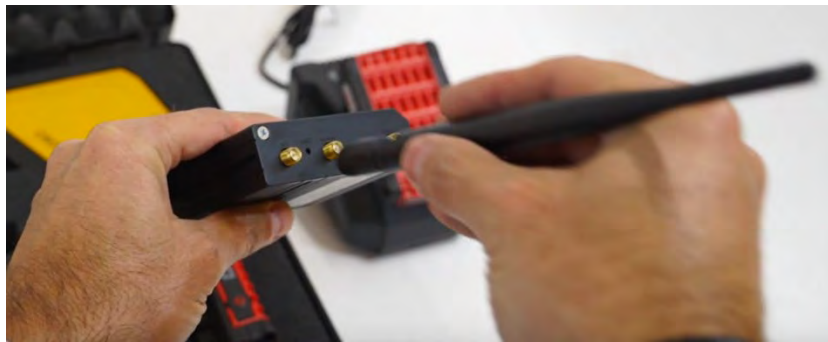
Figure 8: Installation of antennae to the router
