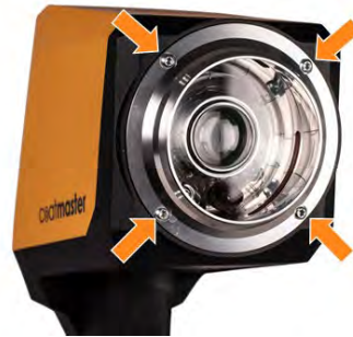
Figure 56: Front glass replacement
